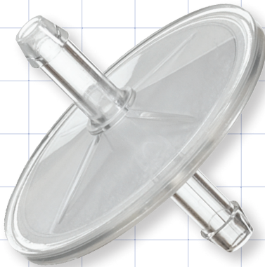
11679 Insufflation Filter with Hose Barb 0.1 Micron 50 mm Diameter, 0.34 inch Hose Barb (8.6 mm) K-Resin, PTFE
