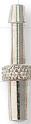
99154 Fits 1/16 inch - 3/32 inch ID Tubing (0.062 inch - 0.093 inch; 1.6 mm - 2.4 mm) Nickel Plated Brass
