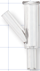
80389 Top Port Female Luer Lock; Side Arm & Bottom Ports 0.079 inch ID x 0.157 inch OD (2 mm x 4 mm) ABS
